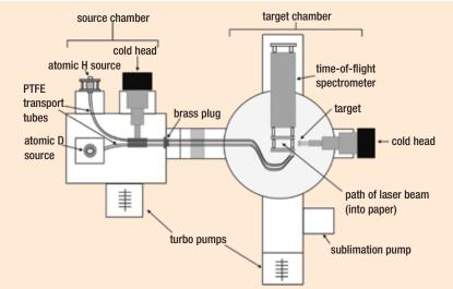
4: A schematic diagram of the UCL experiment to study the formation of H<sub>2</sub> (HD) molecular hydrogen on cold interstellar surfaces using laser spectroscopy. H and D atoms from microwave discharges hit a cooled graphite surface. (Reused with permission from Susan C Creighan, James S A Perry and Stephen D Price 2006 *J. Chem. Phys.* **124** 114701. Copyright 2006, American Institute of Physics)
